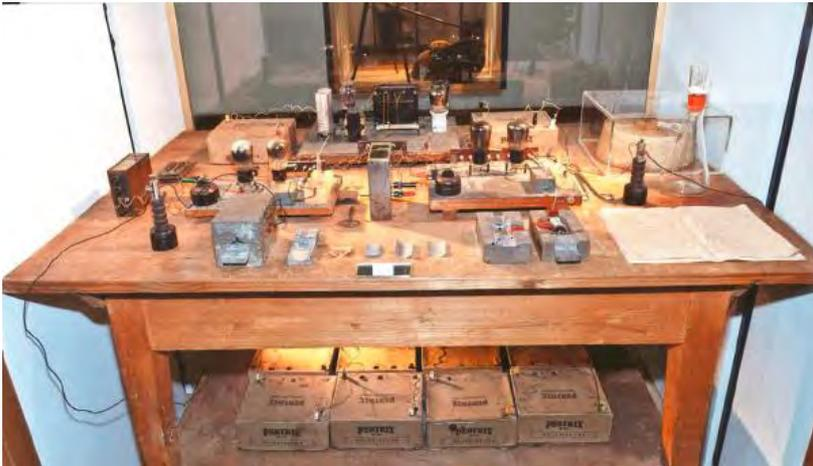
The Hahn-Meitner-Straßmann table shows an arrangement of devices used 75 years ago in experiments which led to the splitting of atomic nuclei for the first time.
